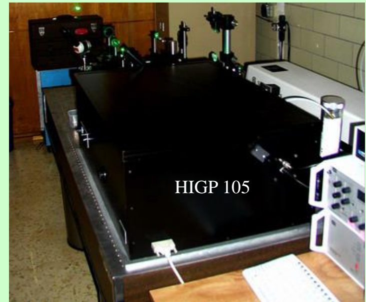
Arrangement for conducting BLS experiments in a DAC
